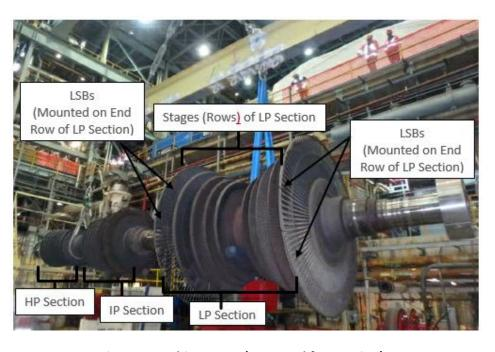
Figure 1: Turbine Rotor (Removed from Unit 1).
